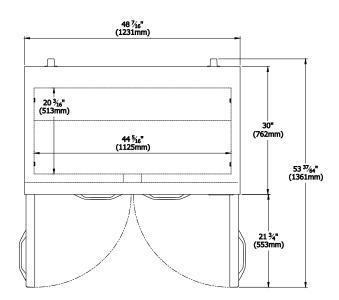
Doors Capacity 13.1 Cu.Ft. Shelves 4 R-290 Refrigerant Temperature 33°F ~ 39°F Range Easy Sliding Condensing Unit Maintenance 9.8 ft long (3m) flexible three Connection wire cord with modeled plug 1/4 HP HP 115V/60Hz Voltage 3.9 **Amps** NEMA 5-15 **NEMA** Config.
