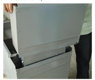
4. Secure it with four self-tapping screws two on the back and one on each side using a 5/16" socket
